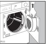
The filter in the inner door must be removed for cleaning.
